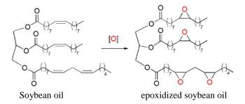
**Fig. 1. Typical epoxidation reaction.** (adopted from Pantone *et al.* 2017)
