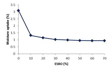
Fig. 8. Effect of ESBO content on the moisture uptake of ESBO/DMU blends
