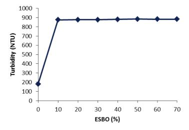
Fig. 7. Effect of ESBO content on the turbidity of ESBO/DMU blends
