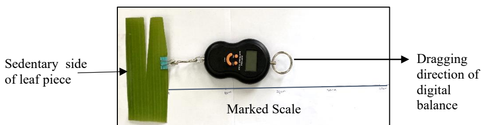
Fig 5: Method designed to measure the tear resistance of plant material
